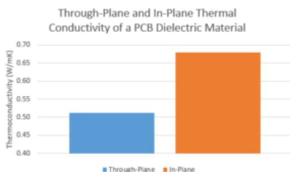
In-plane thermal conductivity of an FR4-type PCB dielectric material
