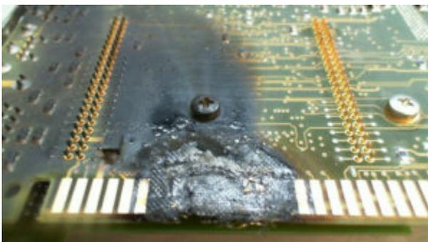
Figure 2. A PCB with a visible failure, caused by overheating. Such a failure can be due to poor thermal management ([Source](#)).
