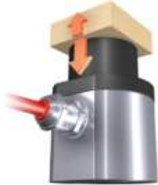
Mathis TCI (Modified Transient Plane Source)
